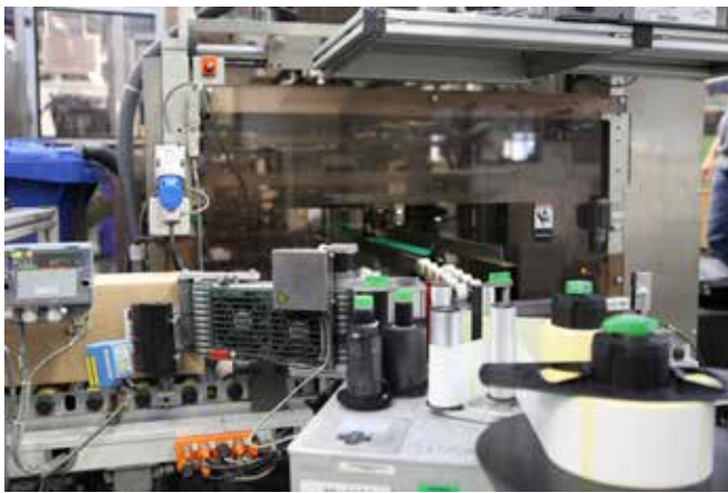
Hermes+ system integrated in a packaging line
